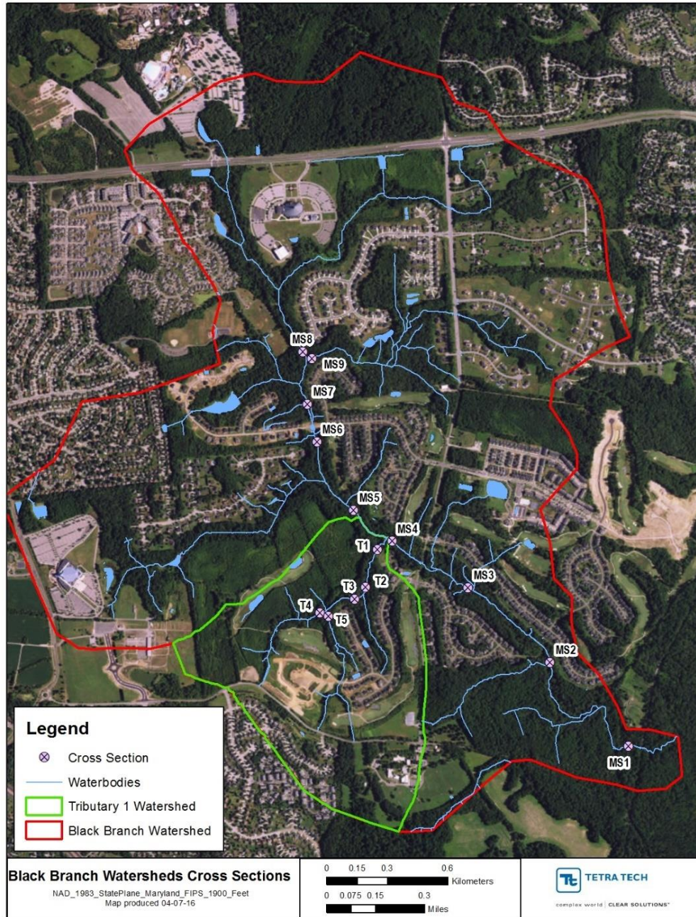
Figure G-2. Locations of Cross Sections in Black Branch and Tributary 1 Watersheds
