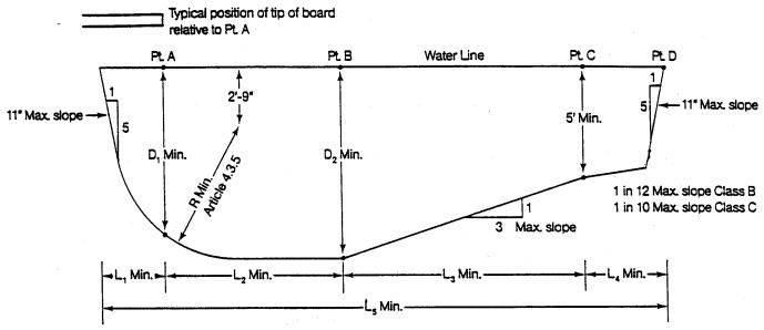
Note: L<sub>4</sub> is a minimum dimension to allow sufficient length opposite the board. This may of course be lengthened to form the shallow of the pool.
