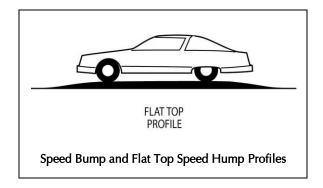
died carefully prior to the installation of any feasible device. The County's experience with flat-top humps has shown they reduce speeds to between 24 and 30 miles per hour (MPH) throughout the entire street.
