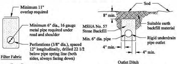
Filter medium allows water to pass through while preventing soil particles from migrating into drainage stone.
