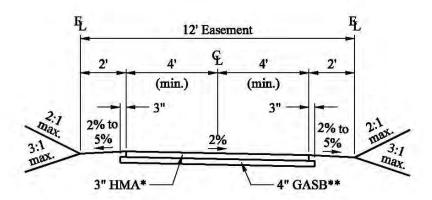
\*3" Hot Mix Asphalt (HMA) surface (fine graduation only). For criteria see Section II, "Technical Specifications." \*\*4" Graded Aggregate Subbase (GASB). For criteria see Section II of these Specifications and Standards and MSHA Standard Specifications for Construction and Materials.
