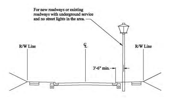
For the required lighting equipment, see the Luminaire and Support Guide for the utility serving the location of construction. (See Section I, Tables I-12 through I-14.)
