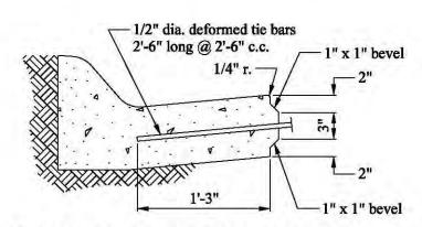
Roll-type Concrete Curb and Gutter - Concrete Pavement
