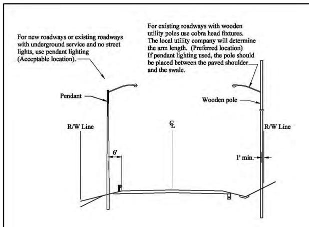
1. For the required lighting equipment, see the Luminaire and Support Guide for the utility serving the location of construction. (See Section I, Tables I-12 through I-14.)
