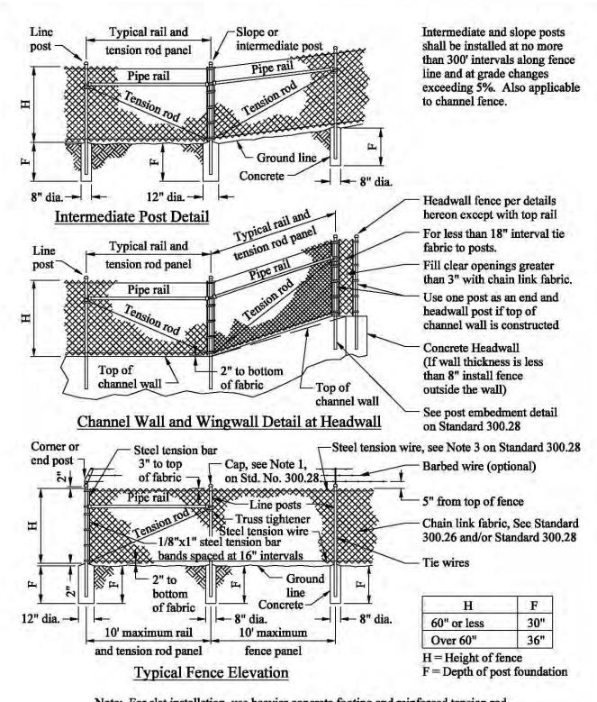
Note: For slat installation, use heavier concrete footing and reinforced tension rod.
