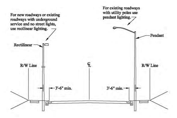
For the required lighting equipment, see the Luminaire and Support Guide for the utility serving the location of construction. (See Section I, Tables I-12 through I-14.)
