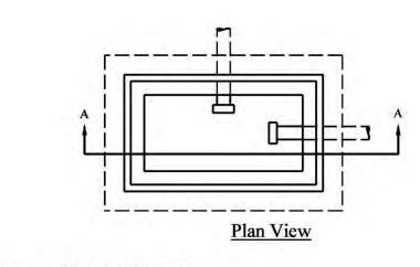
Frame and cover shall be made of high-density polymer concrete, and installed to grade.
