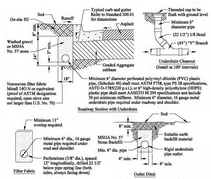
Filter medium allows water to pass through while preventing soil particles from migrating into drainage stone. Exposed pipe at end to be shaped to conform to the terrain along the outfall. An outlet headwall consisting of Class 1 Concrete with No.4 reinforcing bars forming a collar around the pipe may be required in some cases.
