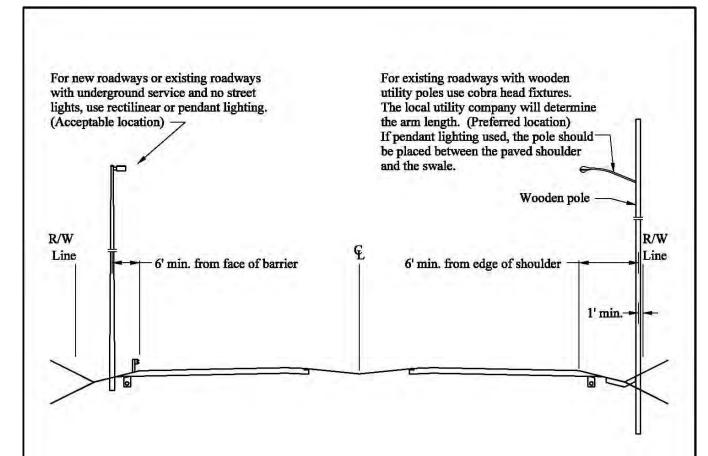
1. For the required lighting equipment, see the Luminaire and Support Guide for the utility serving the location of construction. (See Section I, Tables I-12 through I-14.)
