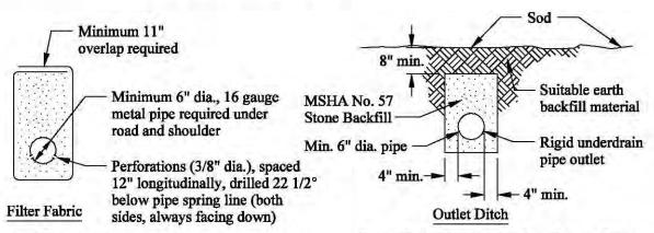
Filter medium allows water to pass through while preventing soil particles from migrating into drainage stone. Exposed pipe at end to be shaped to conform to the terrain along the outfall. An outlet headwall consisting of Class 1 Concrete with No.4 reinforcing bars forming a collar around the pipe may be required in some cases.
