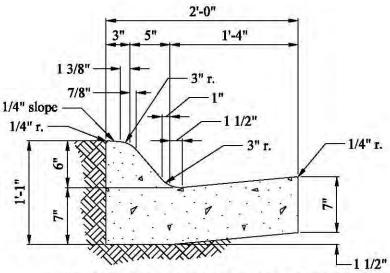
Roll-type Concrete Curb and Gutter - Asphalt Pavement
