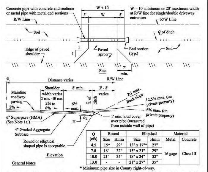
1. Driveway paving section (See Superpave Specifications in Section II of "Technical Specifications; Section 504."):
