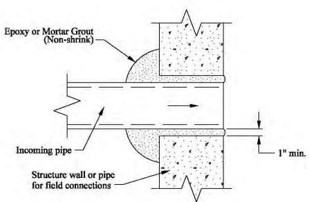
Rigid Plastic Pipe Connection (Minimum 6" diameter pipe)
